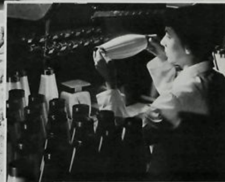
↑ Bobbins of synthetic fibre filament yarn are carefully inspected before they leave the plant for use by Canadian textile mills.
